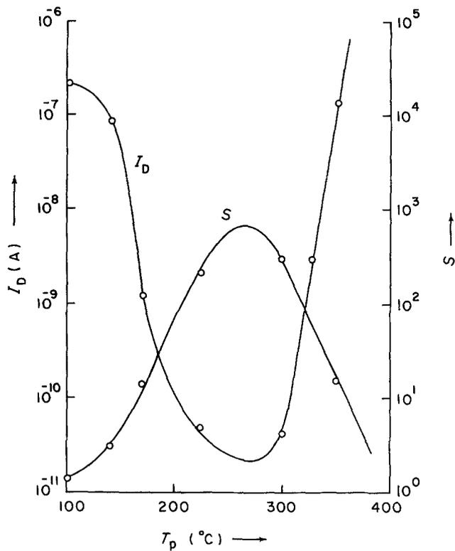
Figure 2 The effect of annealing temperature on dark-condition conductivity ( $I_D$ ) and photosensitivity ( $S$ ).
