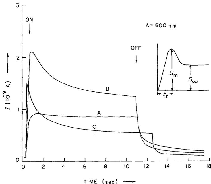
Figure 4 Transient response of photocurrent for samples annealed at various temperatures. Curves A to C correspond to a  $T_p$  of 200, 250 and 300°C, respectively.
