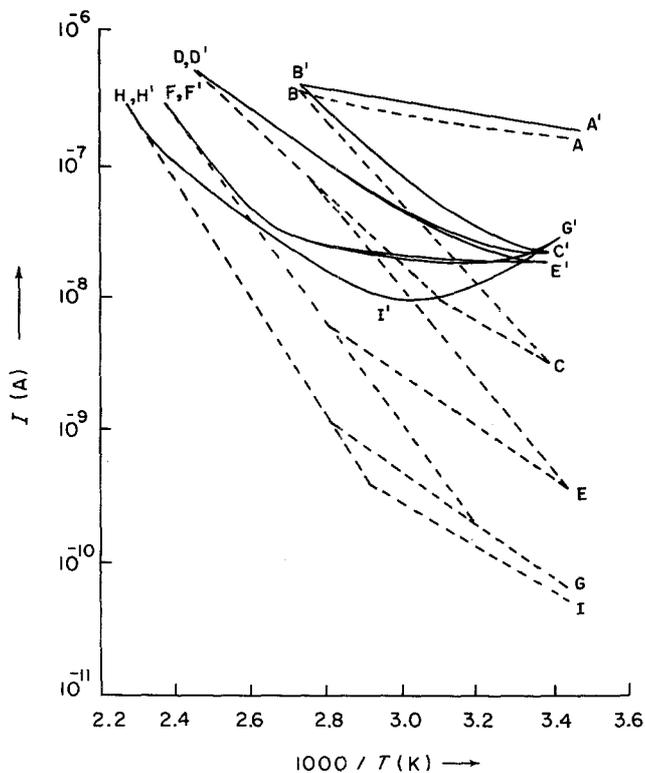
Figure 1 Effect of thermal cycling on  $I_D$  (dotted line) and  $I_L$  (solid line) for five temperature cycles corresponding to a  $T_p$  of 90, 130, 145, 165 and 180°C, respectively.
