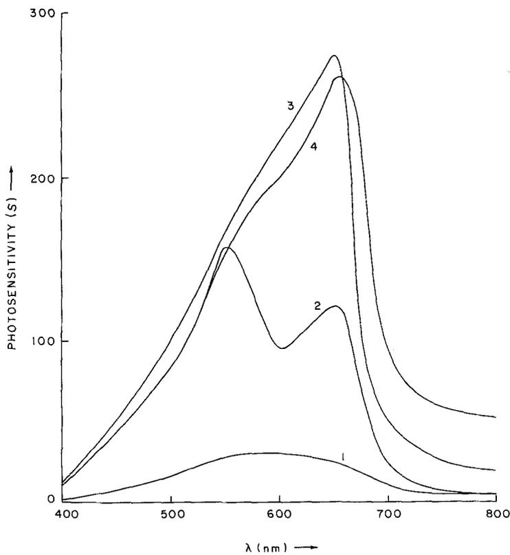
Figure 3 The spectral response of photoconductivity in samples annealed at different temperatures. Curves 1 to 4 correspond to a  $T_p$  of 150, 200, 225 and 250° C, respectively. The photosensitivity is normalized for constant intensity of  $1 \mu\text{W cm}^{-2}$ .
