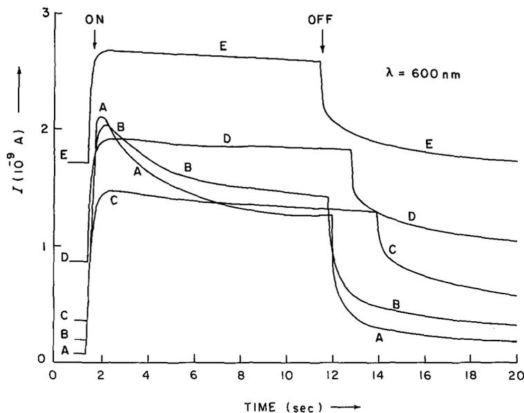
Figure 5 The transient response of photocurrent for the critically annealed sample ( $T_p = 250^\circ\text{C}$ ) at various ambient temperatures. Curves A to E are for temperatures of 20, 35, 45, 60 and  $70^\circ\text{C}$ , respectively.
